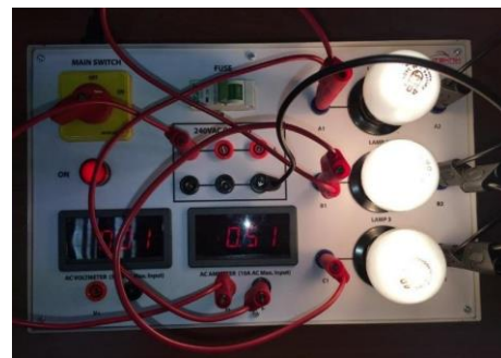
Figure 7: Bulbs are connected in parallel
