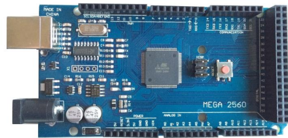
Figure 3: Arduino Mega 2560 R3
