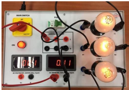
Figure 9: Bulb brightness in series arrangement
