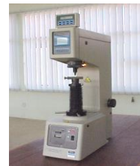
Rajah 5: Mesin Rockwell Model ATK - F3000
